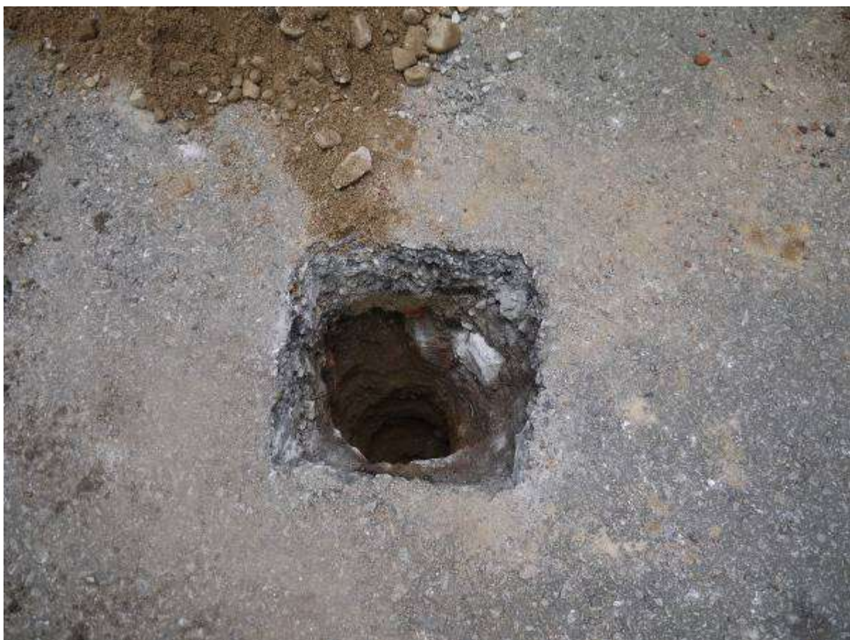
Illustration 40 BH1 test pit 2 totally excavated cobble layer 3 visible in section looking east
