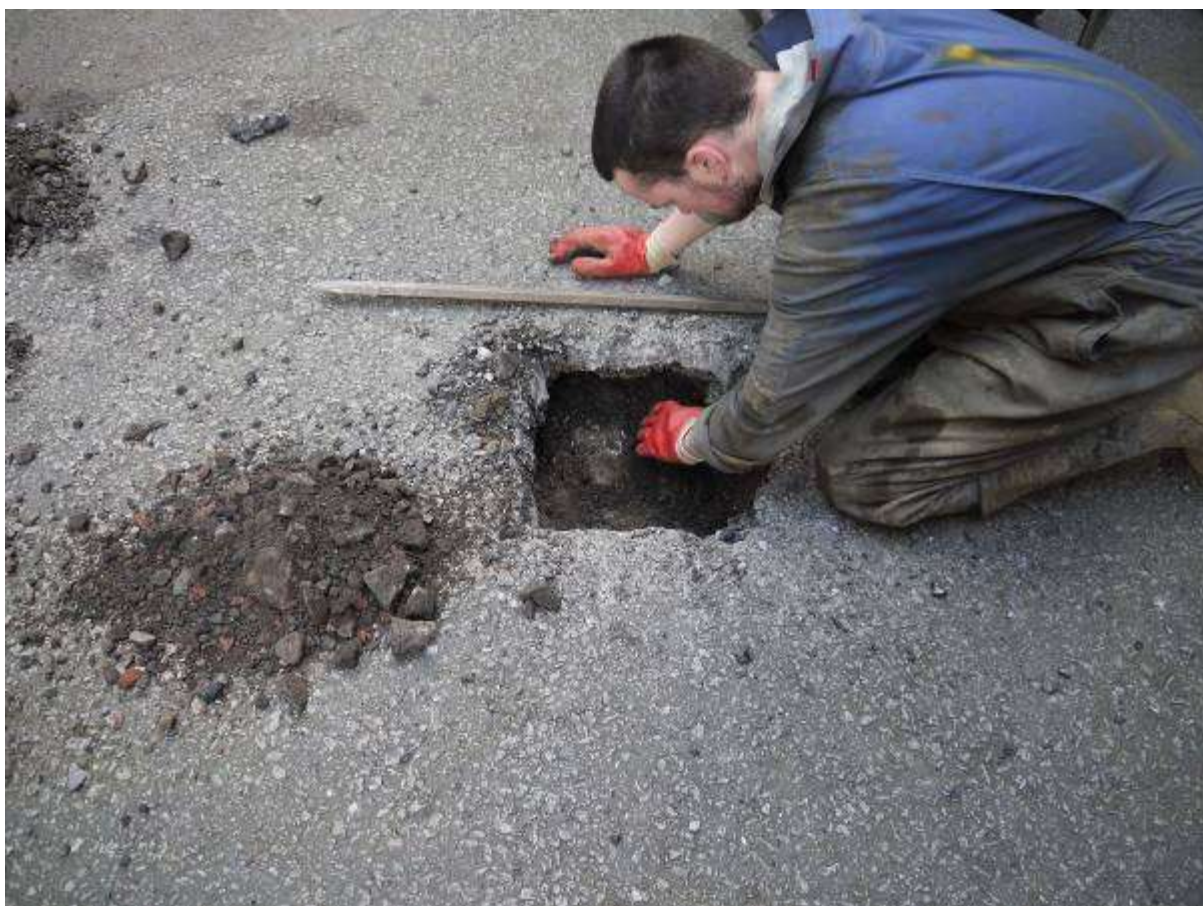
Illustration 39 BH1 test pit cobble layer (3) becoming visible looking east
