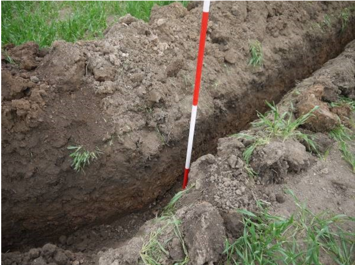
Illustration 12 East facing section of cable trench showing ploughsoil above natural clay at point f on illustration 3
