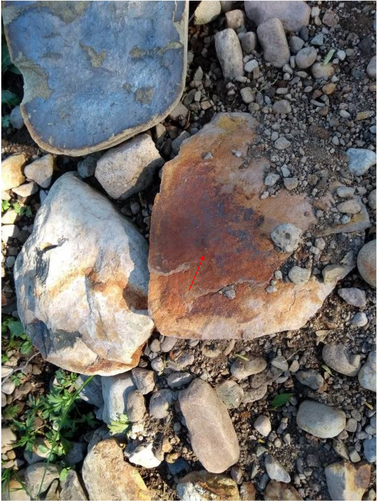
Illustration 8- Typical example of iron panned rock producing metal detector readings (red arrow indicates area of iron pan)
